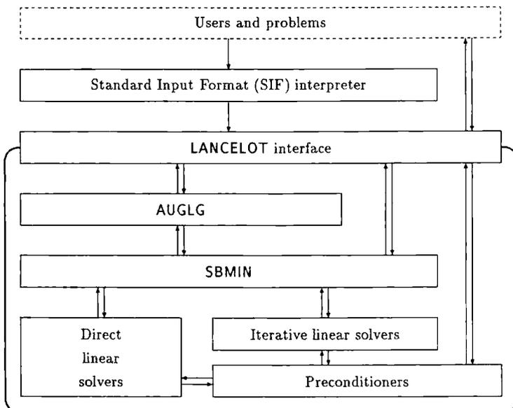
Fig. 1. Structure of the LANCELOT package.
