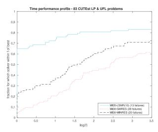
Fig. 16. Time performance profile for LSMR with IC (HSL\_MI35) preconditioning and GMRES(1000) and MINRES with signed IC (HSL\_MI30) preconditioning for test set  $\mathcal{T}$ .
