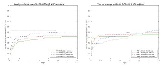
Fig. 8. Iteration performance profile (left) and time performance profile (right) for LSMR with RIF preconditioning using a range of values of localSize for test set  $\mathcal{T}$ .
