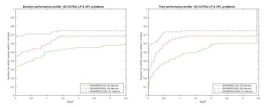
Fig. 9. Iteration performance profile (left) and time performance profile for BA-GMRES with different restart parameters for test set  $\mathcal{T}$ .
