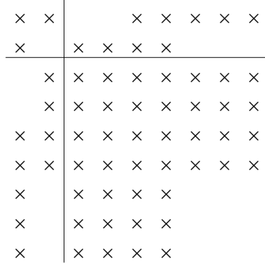
Figure 2.2. A tile pivot, its pivot rows and columns, and fill-in pattern (generated element).
