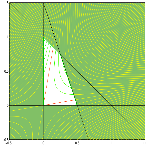
Figure 5.2: Another non-convex problem: contours of the objective function x_1^2 + x_2^2 - 6x_1x_2 and the feasible region for the constraints x_1 + x_2 \leq 1 , 3x_1 + x_2 \leq 1.5 and (x_1, x_2) \geq 0 . Note that escaping from the origin may be difficult!
