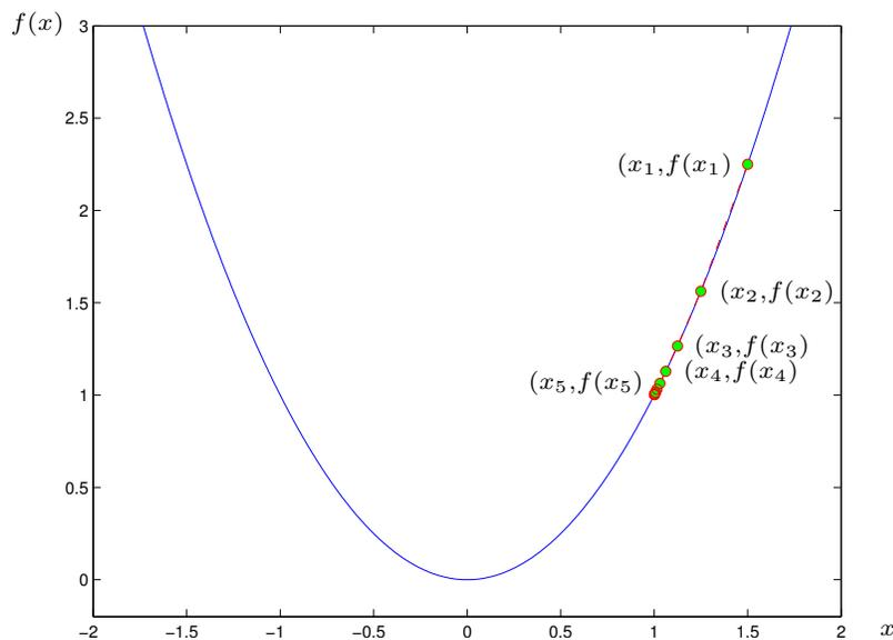
The objective function  $f(x) = x^2$  and the iterates  $x_{k+1} = x_k + \alpha_k p_k$  generated by the descent directions  $p_k = -1$  and steps  $\alpha_k = 1/2^{k+1}$  from  $x_0 = 2$
