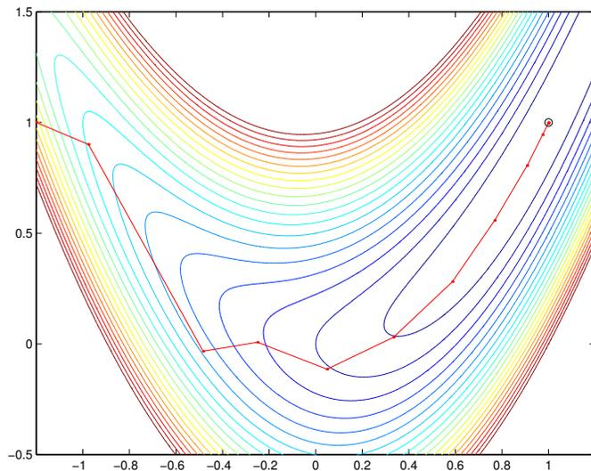
Contours for the objective function  $f(x, y) = 10(y - x^2)^2 + (x - 1)^2$ , and the iterates generated by the Generic Linesearch Newton method
