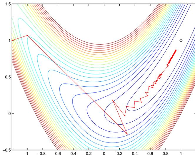
Contours for the objective function  $f(x, y) = 10(y - x^2)^2 + (x - 1)^2$ , and the iterates generated by the Generic Linesearch steepest-descent method
