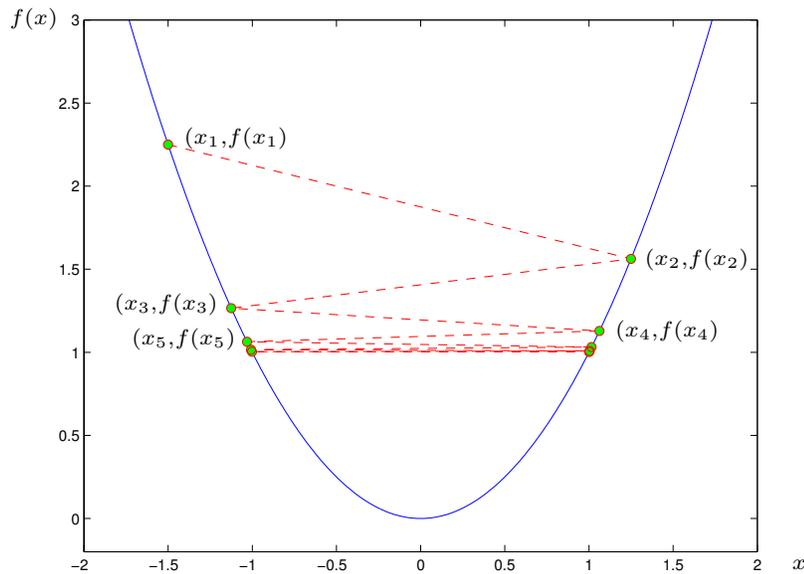
The objective function  $f(x) = x^2$  and the iterates  $x_{k+1} = x_k + \alpha_k p_k$  generated by the descent directions  $p_k = (-1)^{k+1}$  and steps  $\alpha_k = 2 + 3/2^{k+1}$  from  $x_0 = 2$
