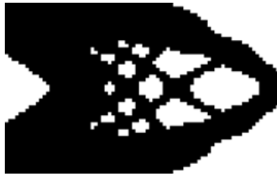
Figure 5. Solution found on mesh of 80 \times 50 elements. The buckling constraint is set to c_s = 0.1 and the compliance constraint c_{\max} = 30 . A volume of 0.692 is attained. Here, the compliance constraint c_1 is active, and the buckling constraint c_2 is not.
