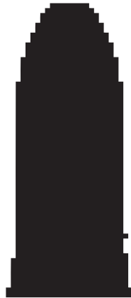
Figure 12. Solution computed on a mesh of 60 \times 60 elements. The buckling constraint is set to c_S = 0.5 and the compliance constraint c_{\max} = 5.5 . In this case, compared with Figure 11, the higher compliance constraint has led to a solution where this constraint is inactive and the buckling constraint is now active.
