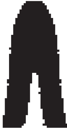
Figure 11. Solution computed on a mesh of 60 \times 60 elements. The buckling constraint is set to c_S = 0.5 and the compliance constraint c_{\max} = 5 . Here, the compliance constraint is active and the buckling constraint is inactive.
