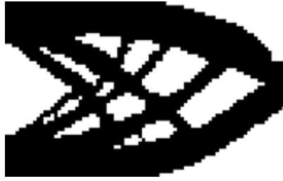
Figure 3. Solution found on mesh of 80 \times 50 elements. The buckling constraint is set to c_s = 0.9 and the compliance constraint c_{\max} = 35 . A volume of 0.6255 is attained. The buckling constraint c_2 is active, and the compliance constraint c_1 is not.
